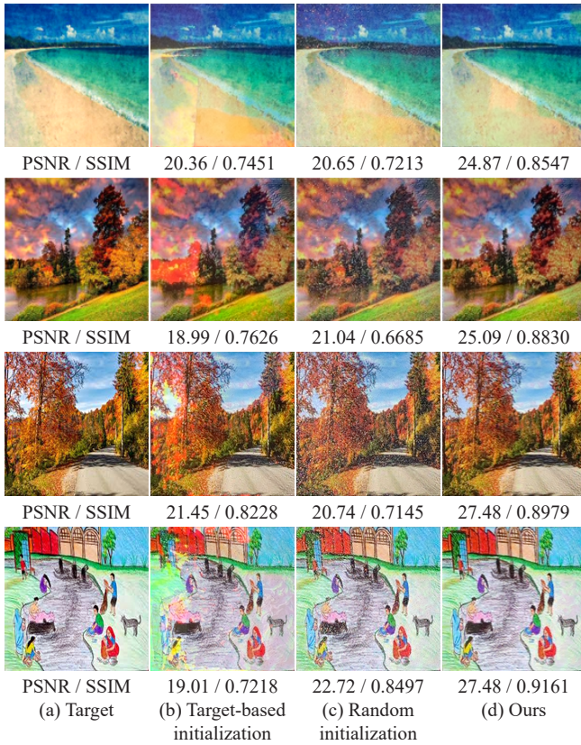
FIGURE 11. Projected outputs of PCDR using different initialization schemes for its optimization. We compare our lighting model-guided initialization (d) with two alternatives: 1) target-based initialization (b) that assigns the projector input directly from the target image (a) and 2) random initialization (c) that sets each texel in the projector input image randomly using a uniform distribution. The surface configurations used in this test are the same as those in Fig. 6. After optimization, alternative initializations result in visual artifacts (b) or residual noise (c). In contrast, PCDR, with our initialization, achieves visually more pleasing and numerically more accurate results.
